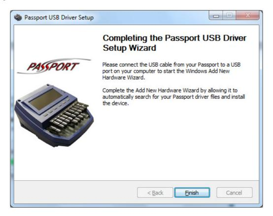
Connect the USB cable from your Passport to a USB port on your computer and turn the Passport on. This should start the Windows Add New Hardware Wizard.
